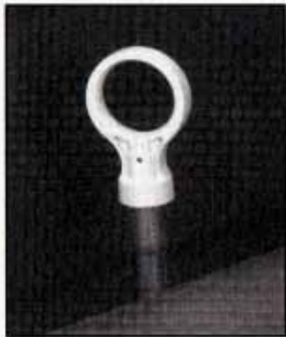
The engine oil dipstick is next to the coolant surge tank. The dipstick handle is a round, yellow loop.
