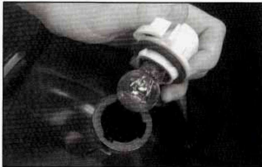
4. Remove the bulb from the socket.
