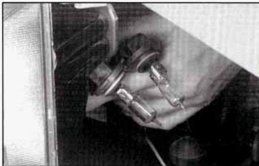
6. Reach behind the lamp and turn the bulb to the left (counterclockwise) to remove it. Don't touch the halogen bulbs. The inner bulb is the high beam and the outer bulb is the low beam.
