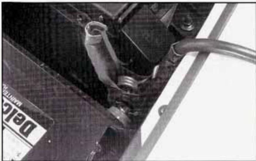
6. Positive (+) goes to positive (+) and negative (-) goes to a metal engine part. Connect the red positive (+) cable to the positive (+) terminal of the vehicle with the dead battery. Use a remote positive (+) terminal if the vehicle has one.
