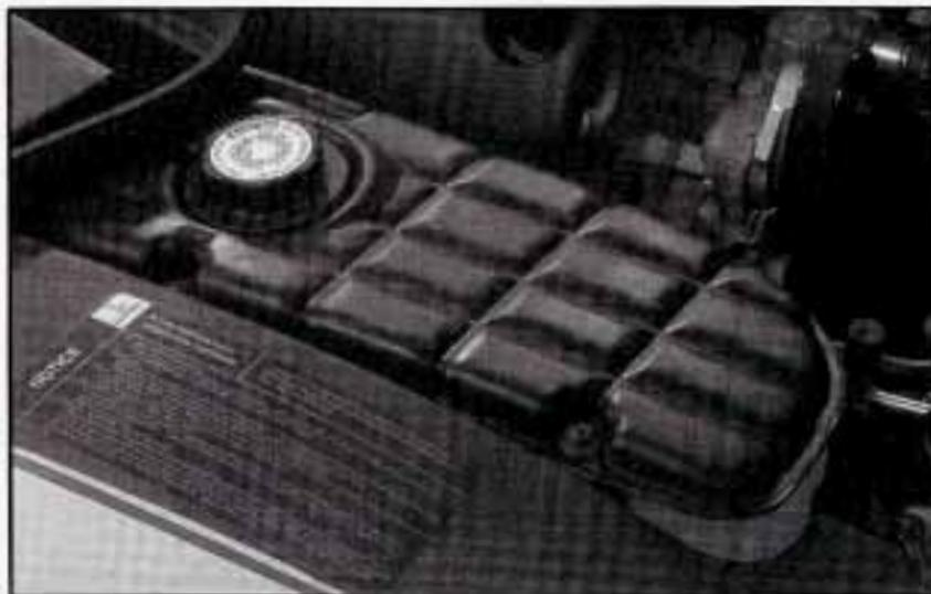
The coolant surge tank is in the engine compartment behind the headlamp.
